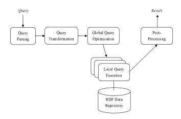
Fig. 3. A distributed query processing workflow
