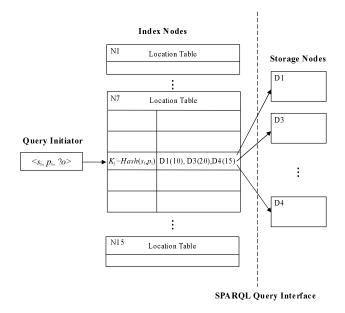
Fig. 2. A Two-Level Distributed Index Structure
