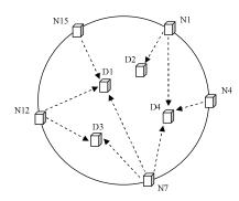
Fig. 1. A peer network of 9 nodes in a 4-bit identifier space
